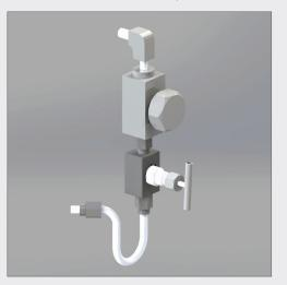
This system includes a thermal relief valve in order to relieve to upstream pressure build up which might occur in the body cavity from thermal expansion. The thermal relief valve automatically operates when the pressure in the body cavity increase of 1.5 Bar (22psi) respect to the pipeline pressure.
