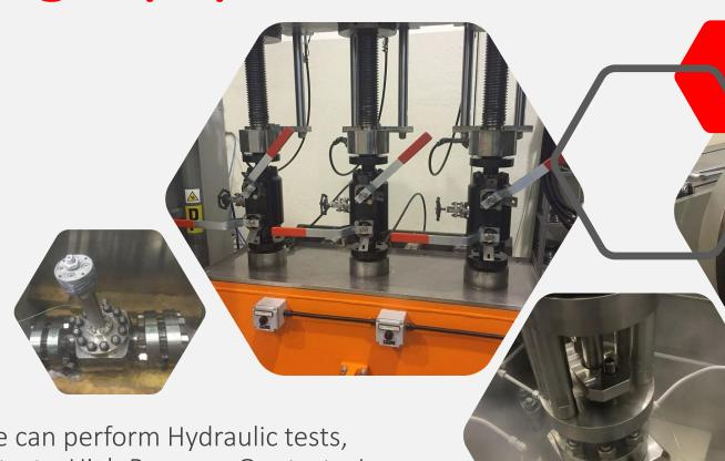
In house we can perform Hydraulic tests, Pneumatic tests, High Pressure Gas tests, Low Temperature tests, Fugitive Emission tests, Torque Tests, Cavity Relief tests, DPE tests.
